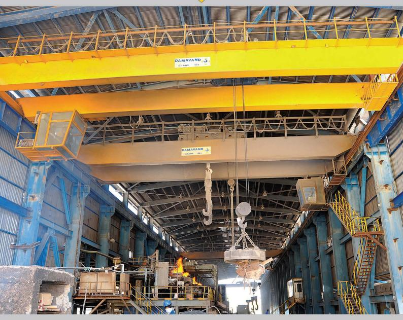
Capacity: 50&16 Tons, class: M7, Span: 24m, for Charging-Teeming.
