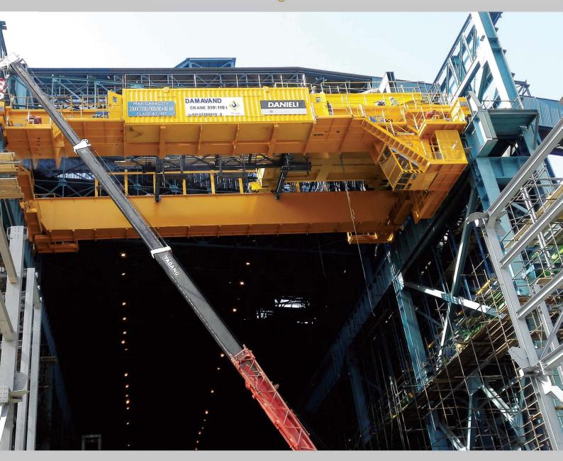
Capacity: 310/110, 270/90 Tons, working class: M7, M8. Span: 23m., Charging-Teeming.
