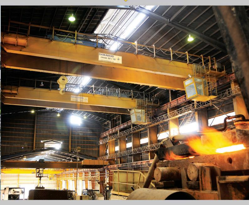
Capacity: 50/15 Tons, class: M8, Span: 25m., for carrying melted materials.
