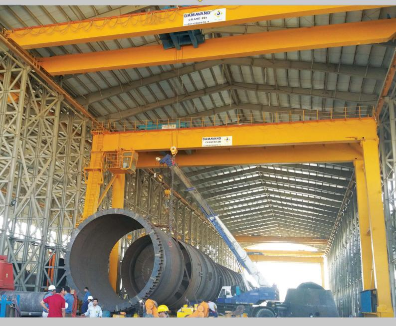
Capacity: Gantry Crane 63/20 Tons, class: M6, Span: 31m, Height: 18m.
